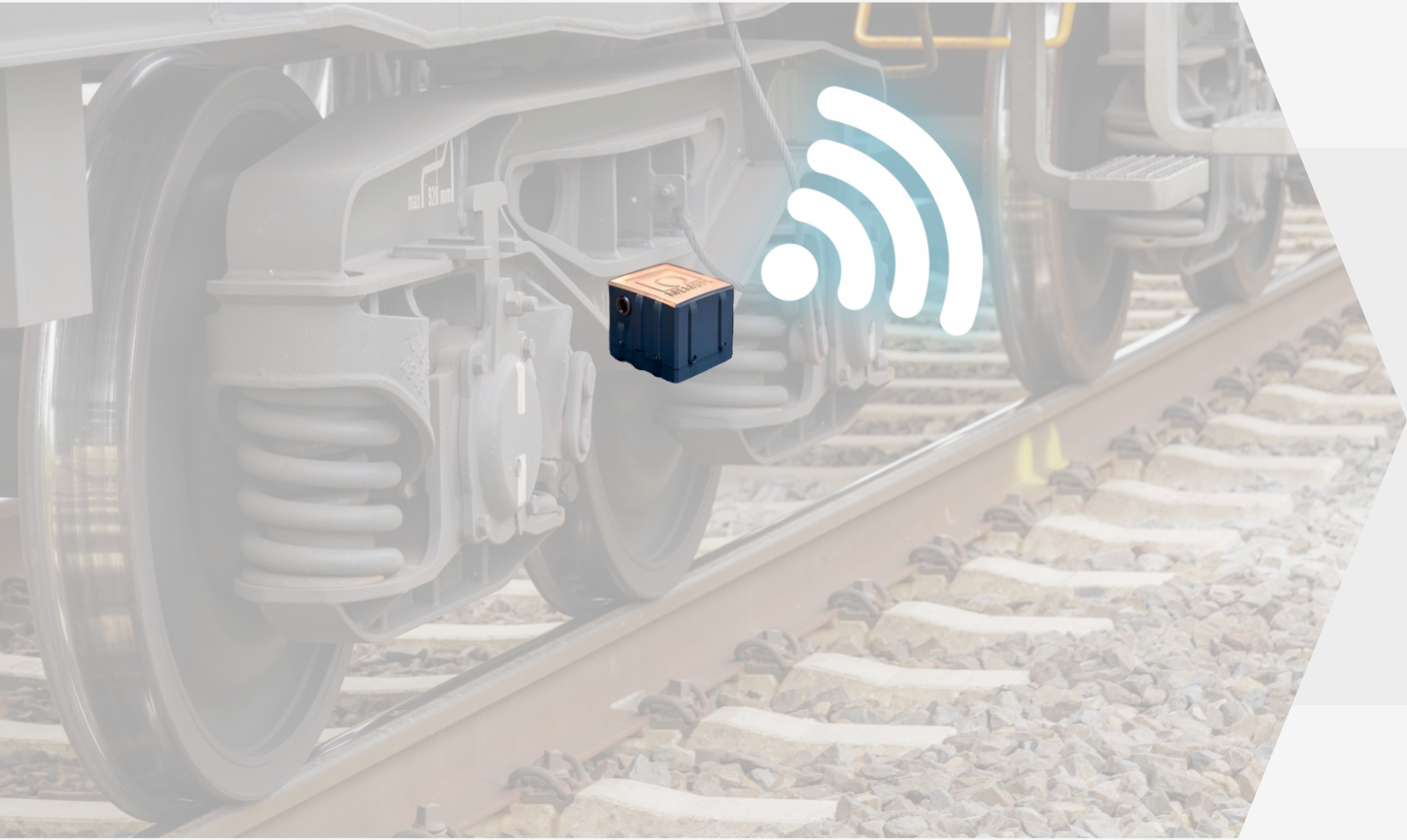
A bogie-mounted IoT module with sensors ...
